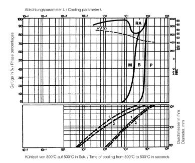
HV10... Vickers Hardness RA... Residual austenite M... Martensite B... Bainite
