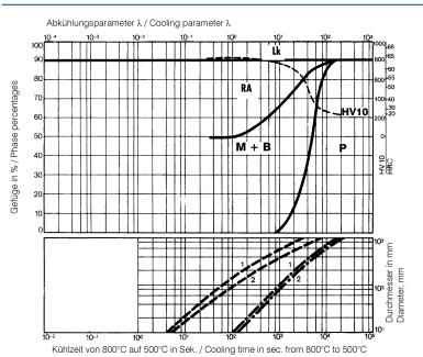
HV10... Vickers Hardness Lk... Ledeburite carbide RA... Residual austenite M... Martensite B... Bainite P... Perlite --- Oil cooling
